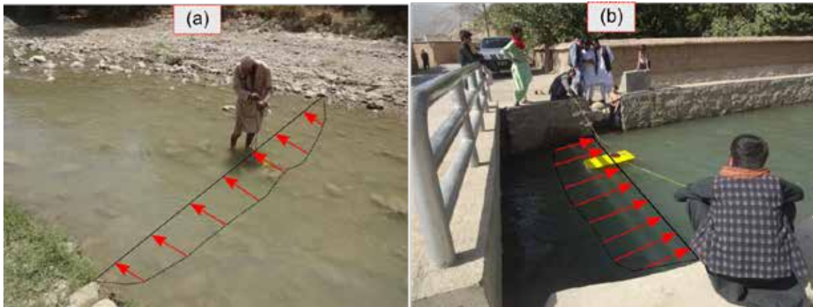
Figure 3.3: Flow discharge measurement for riverbed transmission loss investigation (a) Maidan River using PCM and (b) Khawja irrigation canal in Kapisa province using ADCP device.
